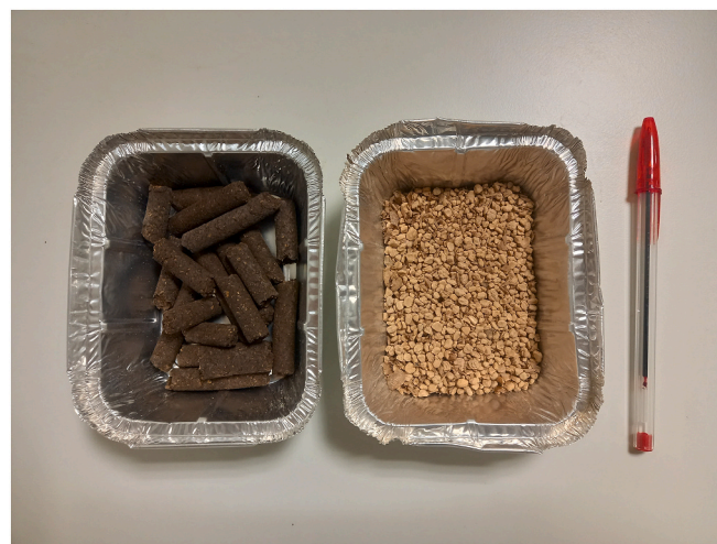
Fig. 2. Samples as received: on the left, exhausted olive cake pellets; on the right, olive stone.
