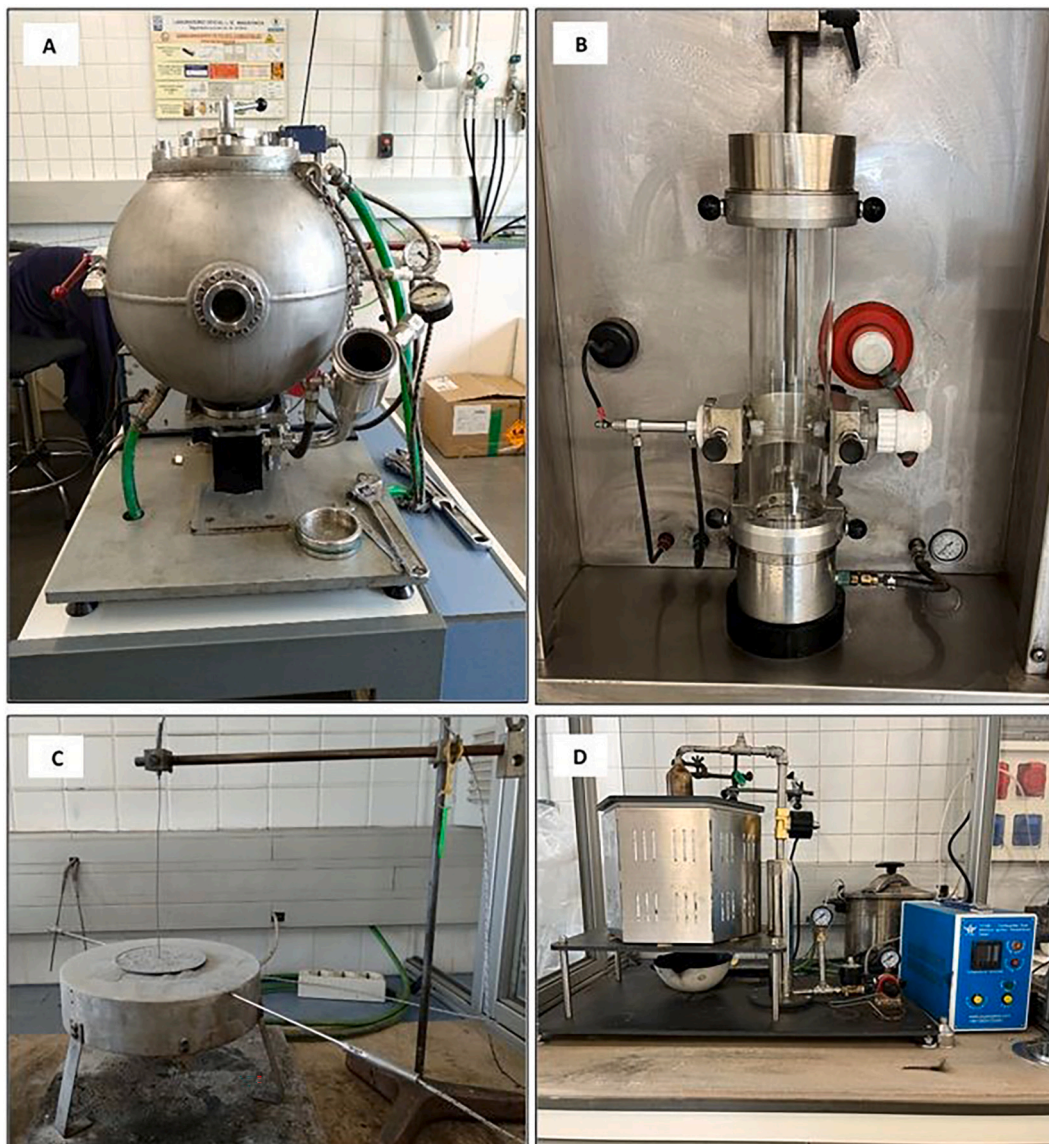
Fig. 3. Laboratory devices for flammability and explosibility tests: 20-L sphere (A), MIKE 3 (B), hot plate (C) and Godbert-Greenwald furnace (D).
